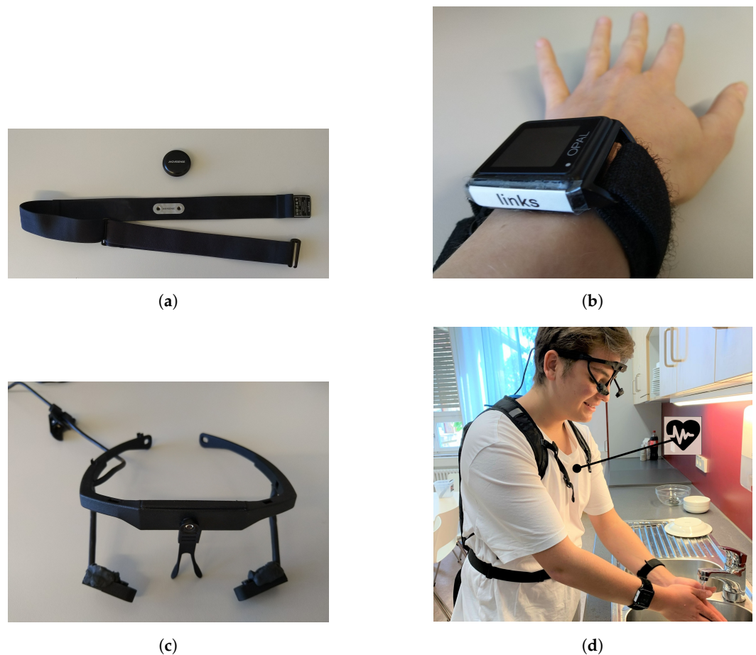
Figure 7. Illustrations of all sensors applied in SKS. (a) Movesense ECG and movement sensor with breast belt. (b) One of two APDM Opal Movement Sensors on the left hand. (c) The 3D printed Look! eye tracker. (d) All sensors at a patient.
